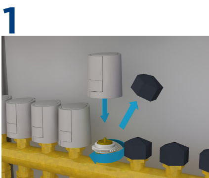
Screw off regulator-caps, screw on the valve adapter, snap on valve drive!
