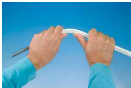
Bending with an internal bending spring
