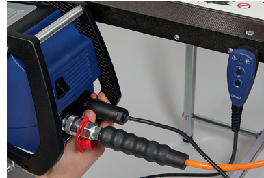
6 Connect the remote control to the back of the pump (push & turn)
