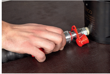
5.2 Connect the female side of the hydraulic line to the pressing chain
