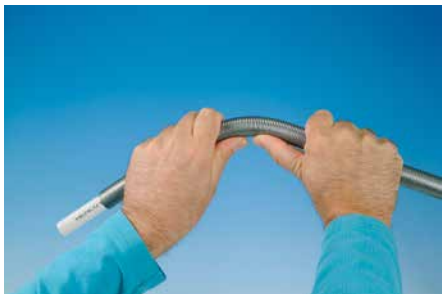
Bending with an external bending spring
