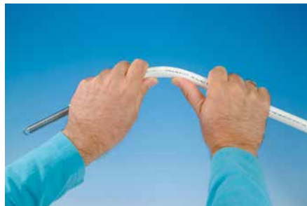
Bending with an internal bending spring
