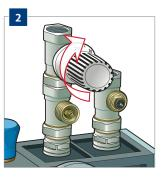
Turn the **RTL knob** to 50. Attach it to the **thermostat valve** by hand and set the parameters in accordance with the district heating supplier's instructions.
