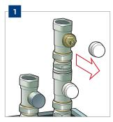
Remove the **protective cap** from the top **thermostat valve**.
