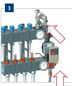
Connect the **filling pipe** to the filling and draining valves, and the **draining pipe** to the return valve (primary side).
