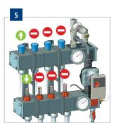
**Fill the first group** by opening it. Make sure that all air is removed from the circuit.
