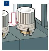
**Reposition the transparent locking cap** to the handwheel to prevent the settings from changing.
