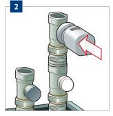
Attach the **zone valve** to the **thermostat valve** by hand.
