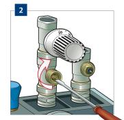
Close the **return valve** using a screwdriver.
