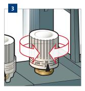
Set the calculated flow by turning the **hand wheel** to the desired value.
