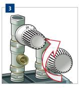
Turn the **thermostat knob** to 6 and connect it to the **thermostat valve** by hand.
