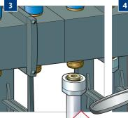
Connect **the underfloor heating pipe** to the **return distributor**.
