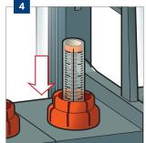
**Reposition the red cap back** over the flow meter to prevent the settings from changing.
