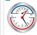
**Pressurize the distributor.** Minimum 4 bar, maximum 6 bar (in accordance with NEN-EN 1264-4 guidelines).
