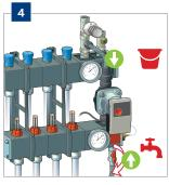
**Open** the filling and the draining valves.
