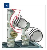
Adjust the **RTL knob** in accordance with the district heating supplier's instructions. Set the return temperature by turning the knob to the desired value(s) and lock this value/these values by using the two pins provided.
