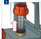
Remove the the **red cap** from the flow meter.
