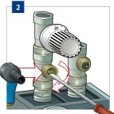
**Connect the return valve** using a screwdriver and screw the provided hose nipple to the return valve.
