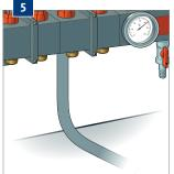
**Install the pipe.** Avoid tension on the distributor by making a perpendicular, but fluid curve.
