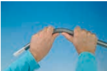
Bending with an external bending spring
